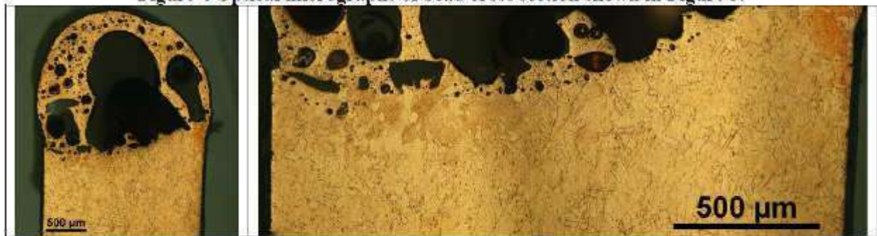
Figure 4 Optical micrographs of bead cross section shown in Figure 3.
